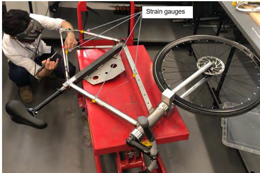
Figure 11: Image of the frame during strain gauge welding, showing strain gauge sites.
