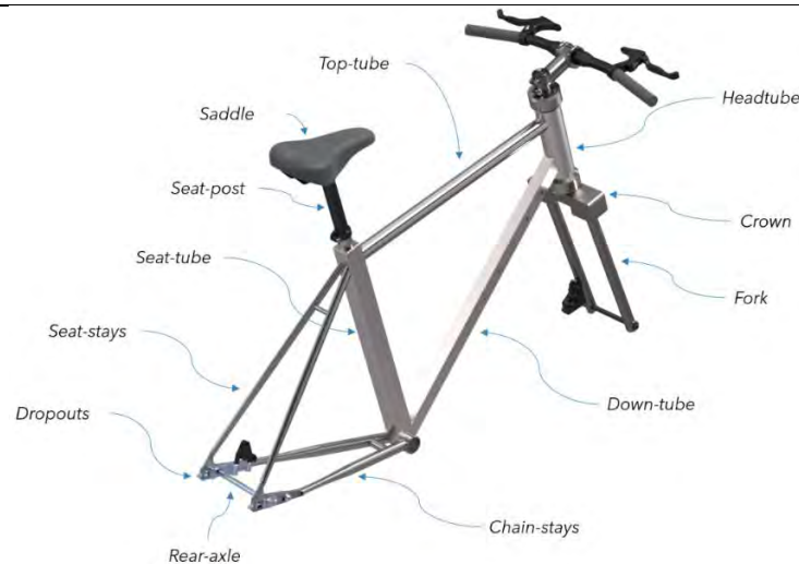
Figure 1: General terminology for frame components.
