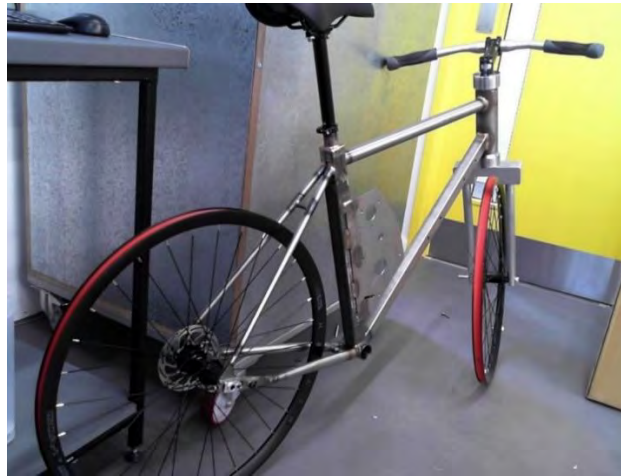
Figure 6: The frame with the Aluminium thru-axle as designed by the group in the front wheel.
