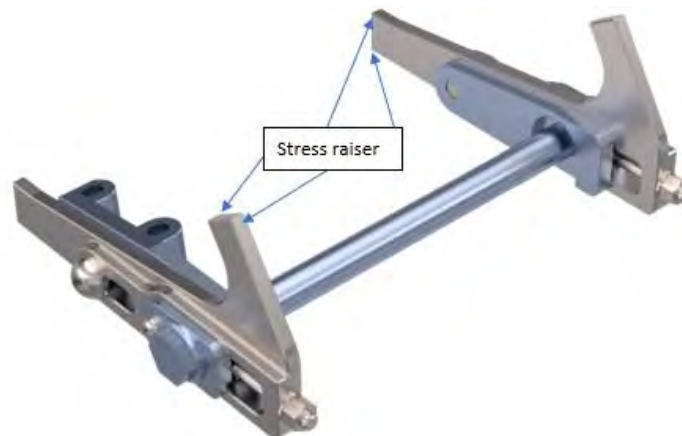
Figure 30: Current full rear dropout assembly.
