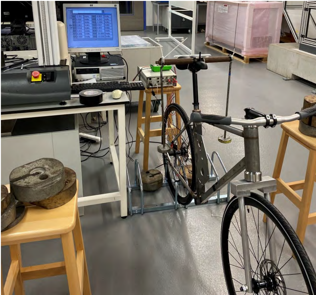
Figure 16: The bike as set up for testing with the Madaq voltage values on the screen.
