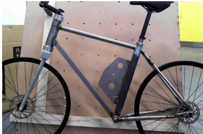
Figure 5: The frame and steering fork assembled for testing.
